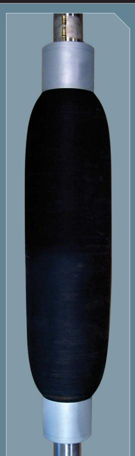
RST Instruments Borehole Packers are pneumatically or hydraulically inflatable packers that incorporate one fixed and one sliding head attached to a center shaft. This sliding head allows the packer gland to retract about the center shaft as it inflates.
