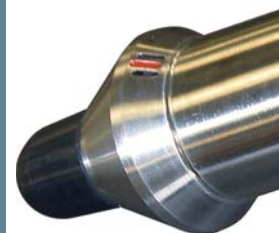
Close up of tip showing top (centre) reference markings which are used for proper orientation during operation.
