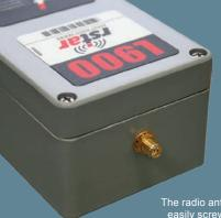
The radio antenna can be easily screwed into the connector which is at the top of the DT2011B case.
