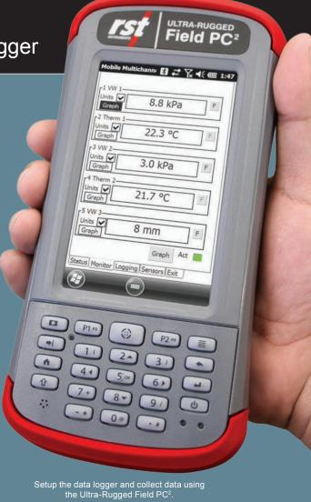
Screenshot of DT2055B Mobile software as shown on the Ultra-Rugged Field PC<sup>2</sup>.
