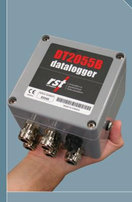
The DT2055B Ten Channel Data Logger is a low cost, battery powered data logger, designed for reliable, unattended monitoring of up to 10 sensors which may be any mix of vibrating wire sensors and thermistors, typically 5 vibrating wire sensors with their associated thermistors.
