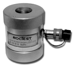
After saturation of the pressurization chamber, the cylindrical rock sample is inserted into the chamber within the confining membrane. The two spherical seats are positioned so that the rock core lies centrally in the triaxial chamber.
