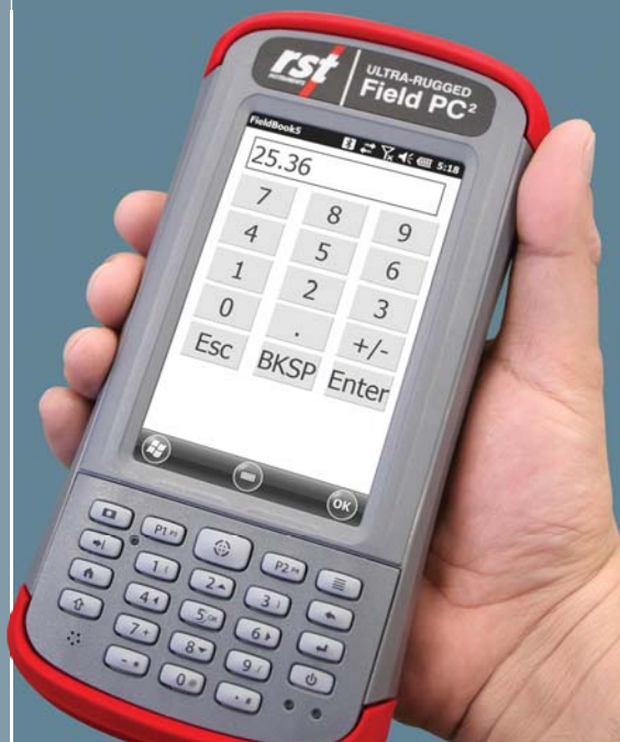
Water level readings being manually entered into FieldBook at a project site.
