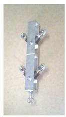
tubing, generally installed within installation time. drilled hole, used а in conjunction with a wheeled sensor probe system determine sub-surface ground dynamic movements. internal grooves provide an orientation reference for the inclinometer probe readings. attention is paid to minimise the twisting of the casing grooves.
