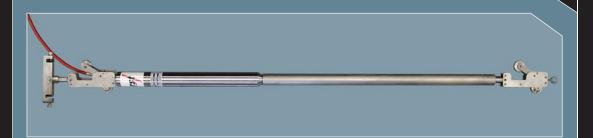
The Horizontal In-place MEMS Inclinometer is designed to remotely monitor, and continuously measure, underground vertical movement as a result of construction and excavation and any settlement that may occur around tunnels, dams, embankments and landfills.
