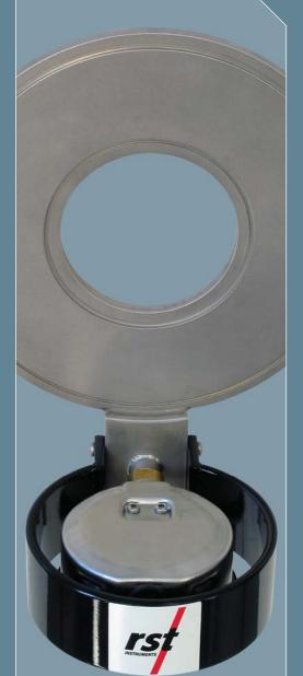
Hydraulic Load Cells are constructed from stainless steel. The load is distributed equally over the loading area of the cell by a thick, machined steel distribution plate. The load, when applied to the cell, causes a pressure increase in the hydraulic fluid, and this change in pressure may be measured via a Bourdon Tube Gauge or a variety of electrical transducers.
