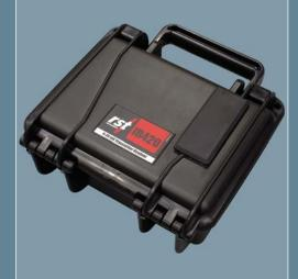
The IR420 reads, displays, logs and powers 4-20 mA transmitters
