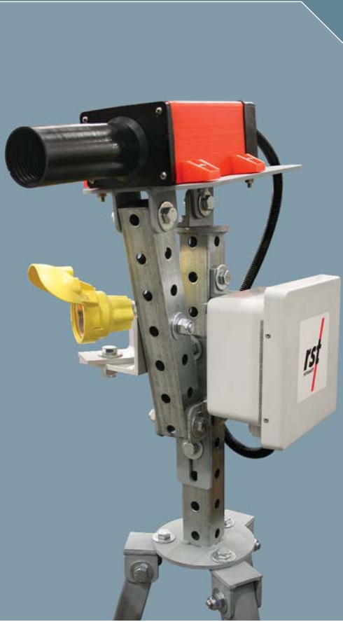
Close-up of portable precision laser distance meter mounted on top of tripod with accompanying RST datalogger.
