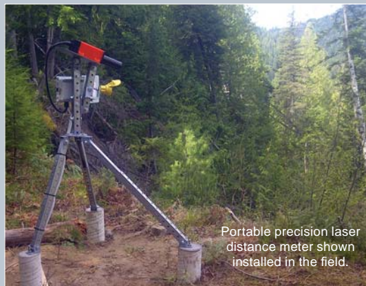
A portable precision laser distance meter shown mounted on a tripod base.
