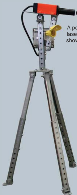
Shown with attached survey reflector to enable survey tie-in of the instrument.
