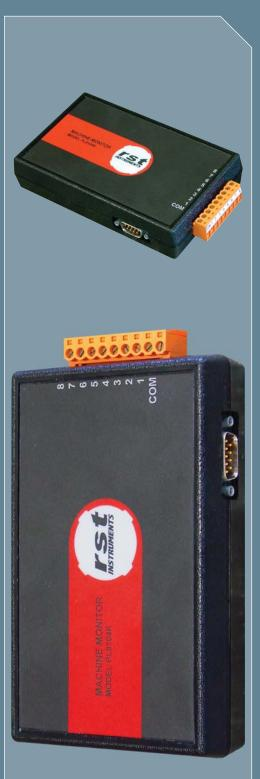
The RST Machine Monitor System can monitor up to 8 pumps simultaneously. Data is collected whenever a pump's status changes for more than a one second interval.
