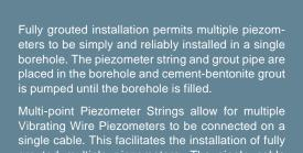
grouted multiple piezometers. The single cable prevents vertical void channels. Tough urethane jacketed, Kevlar® reinforced, non-stretch cable is employed to withstand the rigors of installation and is entirely water-blocked to minimize any leakage. No conductors are shared to maximize independent reliability of each sensor.
