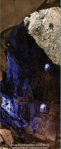
RST's Paste Backfill Monitors are used in mine paste backfill to achieve improved extraction and to increase safety. They provide useful engineering feedback to allow paste and stope design to be
