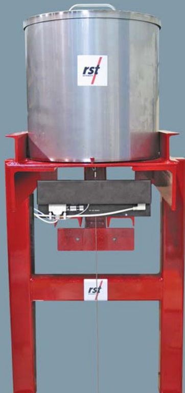
Inverted Pendulum shown with RxTx Teledendum.
