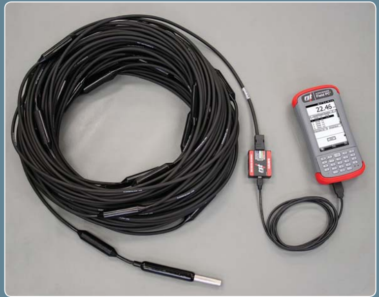
Thermistor String shown connected to the Ultra-Rugged Field PC 2 for direct reading.
