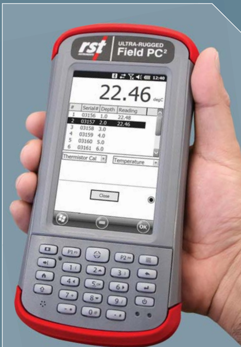
Ultra-Rugged Field PC 2 showing direct node readings.
