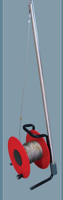
RST Well Sounders are designed to measure the depth of boreholes, standpipes and wells. RST Well Sounders employ a high accuracy, non-stretch, stainless steel wire marked in standard 10 ft. graduations that are clearly stamped on to sturdy brass crimps. Alternate graduations are available to user specified requirements which must be requested at time of ordering.
