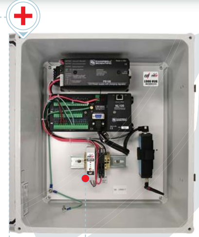
A flexDAQ enclosure shown with an open lid to reveal an installed RSTAR L900 RTU (on DIN rail), datalogger, radio and power supply.
